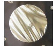
500nm Zr foil mounted "loosely" on TF111-frame. 13nm photons, 300 pulses x >5 \mu /pulse x 1 \mu sec interval, 1mm diameter (discoloration, no hole)
