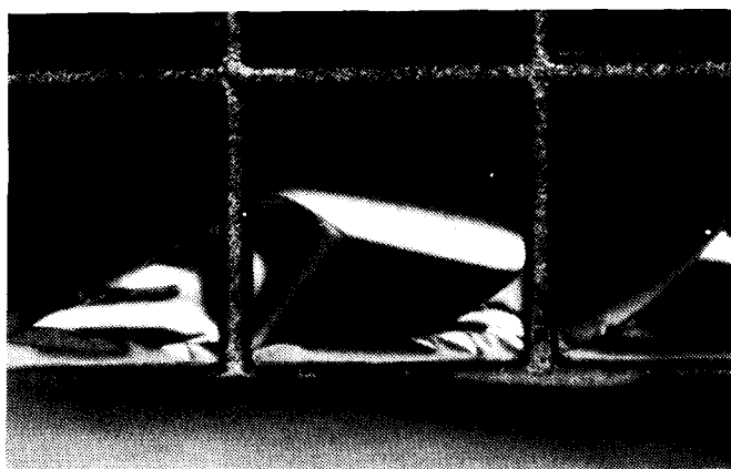
Figure 5. Front lit photo of damaged filter (Mesh “pane” size is 0.0143 in.)
