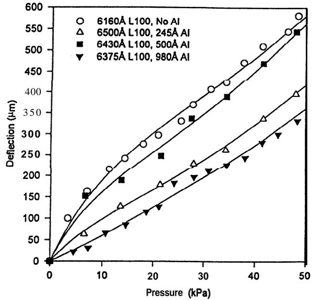
Figure 6. Deflection vs. pressure for polyimide near 6400Å thick with various thicknesses of Aluminum
