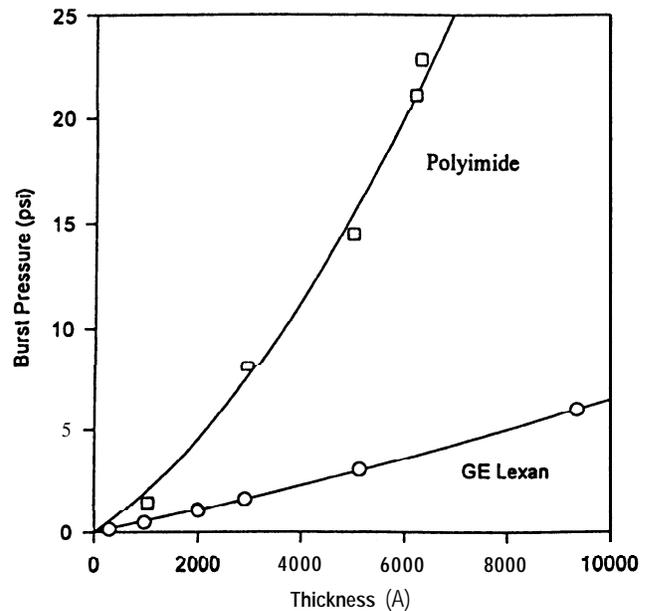
Figure 3. Burst pressure vs. Thickness for Lexan and polyimide
