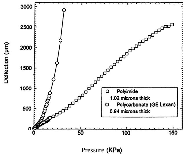
Figure 2. Deflection vs. Pressure for Lexan and polyimide
