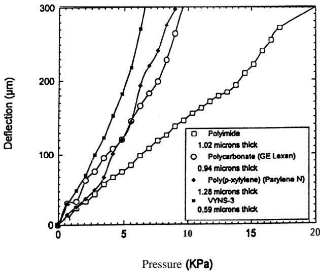
Figure 1. Deflection vs. Pressure for various polymers
