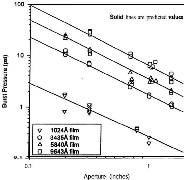
Figure 4. Burst pressure vs. Aperture size for various thicknesses of polyimide
