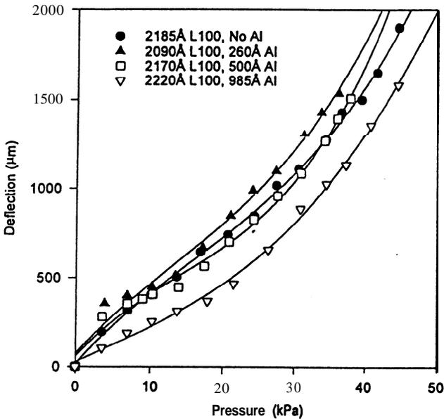
Figure 5. Deflection vs. Pressure for polyimide near 2 100Å thick with various thicknesses of Aluminum
