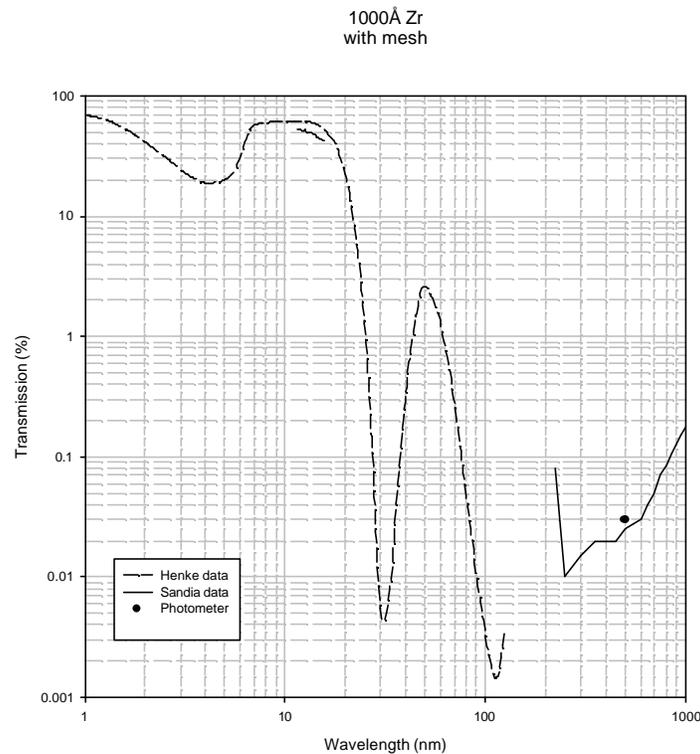
Figure 1. ETS Filter Transmittance vs Wavelength
