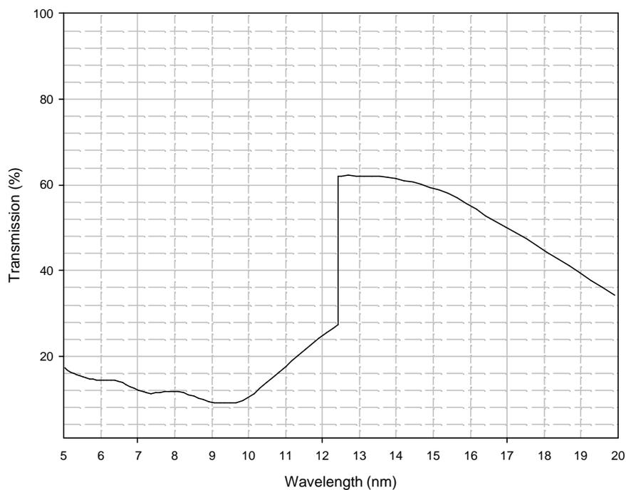
Figure 2. Si/Zr/Si filter transmittance vs wavelength
